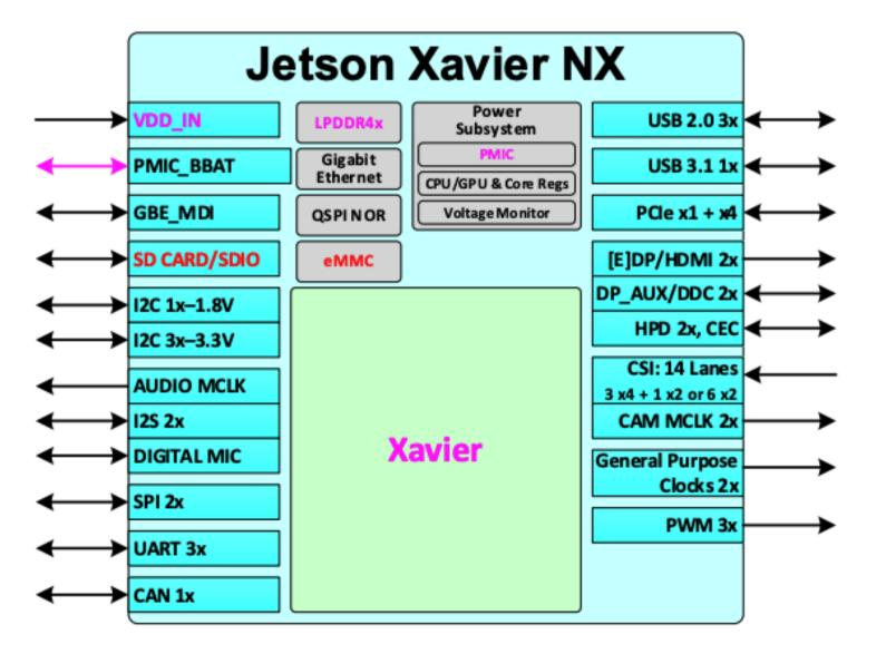
The interfaces or blocks that are supported only by one of the modules is highlighted in red.
